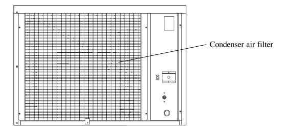
2. Remove the condenser air filter with a screwdriver.
